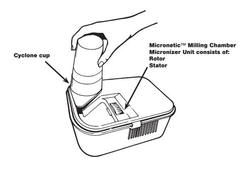
Turn the mill upside down and attach the cyclone cup to the bottom of the mill. Align the handle of the cup in the position shown. Be sure to empty the cyclone cup after each milling session. Any flour you find in the cup is perfectly good and should be used. The function of the cyclone cup is to separate the flour from the air as it passes through the mill.
